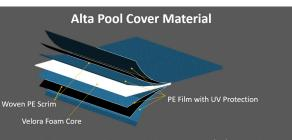
Constructed Of A Closed Cell Cross-linked Polyethylene (PE) Foam That Is Laminated On The Top And The Bottom With A Woven PE Scrim. This Scrim Is Coated Top And Bottom With 2 mils Of PE Film and UV Stabilizing Additives.
